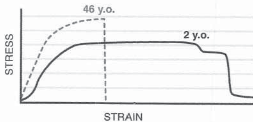
FIGURE 39-1 Stress-strain curves for mature and immature bone. The increased strain of immature bone prior to failure represents plastic deformation. (From Rang M: Children's Fractures. Philadelphia, JB Lippincott Co, 1983. Originally from Currey JD, Butler G: The mechanical properties of bone tissue in children. J Bone Joint Surg 1975;57-A:810.)
